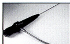
Needle scope with light guide cable
